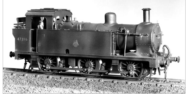
**Prototype.** Fowler designed this class of locomotive as the LMS standard shunting and general-purpose tank. 422 members of the class were built. They were often used for local passenger trains and some were fitted for push-pull working. Some of the class lasted to the end of steam and a number are preserved.
