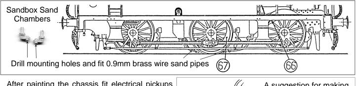
After painting the chassis fit electrical pickups and motor/gears and set up for sweet running.
