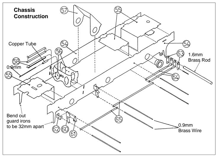
**Parts 54, Chassis Sides.** Emboss rivet detail then open out bearing holes with a tapered reamer.
